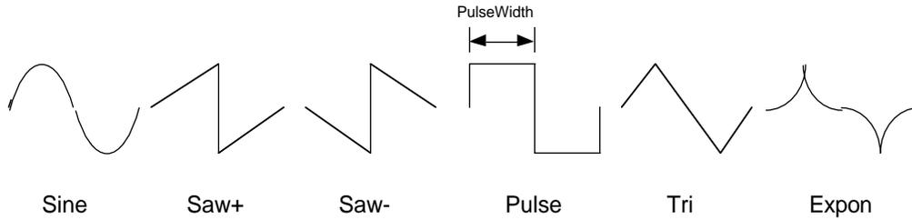
**Figure 10-61 Configurable Wave Shapes**
