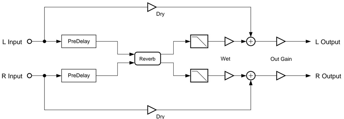
**Figure 10-5** Simplified block diagram of Stereo Hall.
