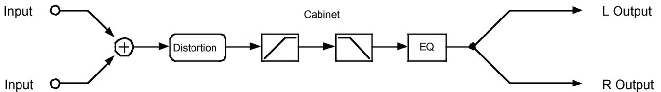
**Figure 10-35** Block diagram of MonoDistort + EQ
