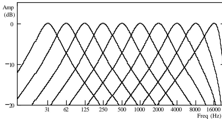
**Figure 10-96** Filter Response of Each Bandpass Filter
