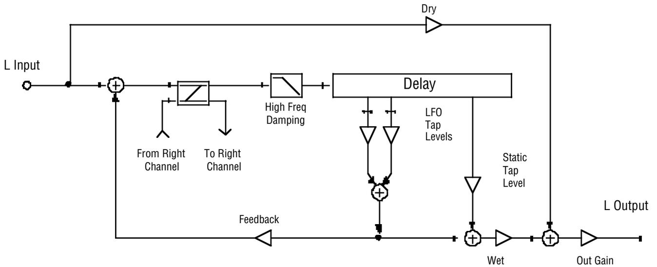
Figure 10-17 Simplified block diagram of the left channel of Flanger 1 (right channel is similar)
