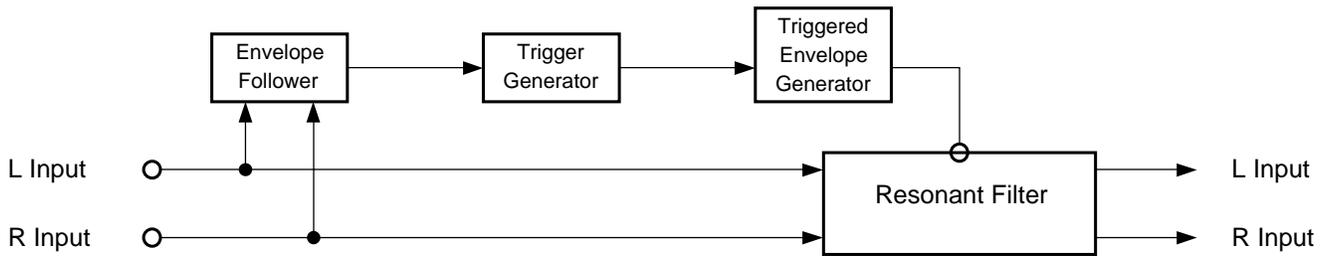
**Figure 10-52** Block diagram of Triggered Envelope Filter
