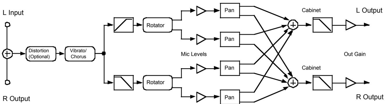
**Figure 10-40** Block diagram of VibChor+Rotor
