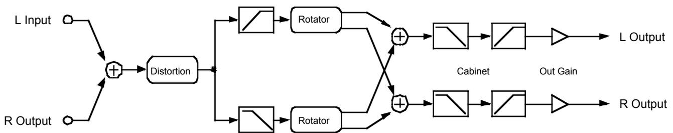
**Figure 10-43** Block diagram of Distort + Rotary
