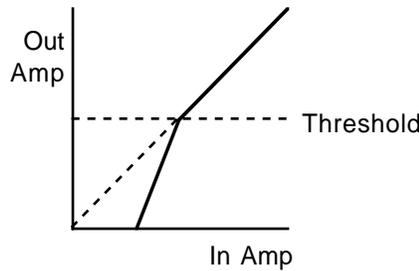
**Figure 10-78 Expansion Transfer Characteristic**
