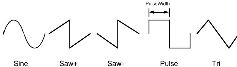
**Figure 10-54 Configurable Wave Shapes**
