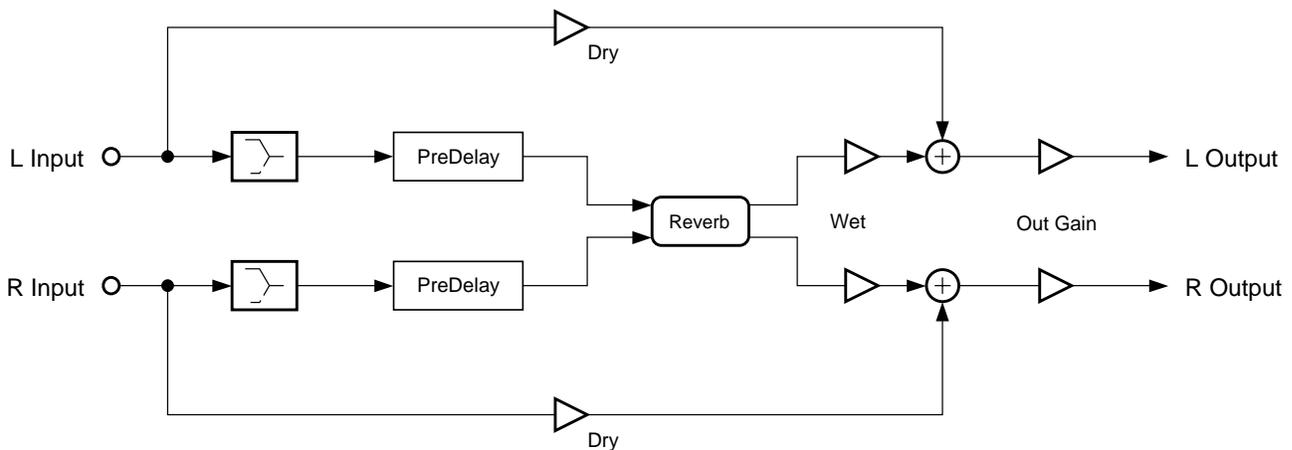
**Figure 10-4** Simplified block diagram of Panaural Room.
