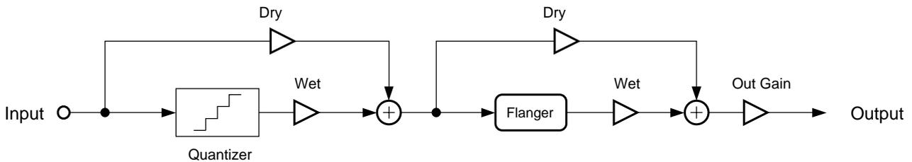
**Figure 10-31** Block diagram of one channel of Quantize+Flange.
