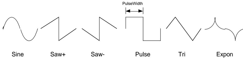
**Figure 10-93 LFO Shapes available for Dual AutoPanner**
