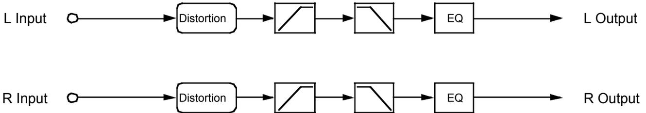
Figure 10-36 Block diagram of StereoDistort+EQ
