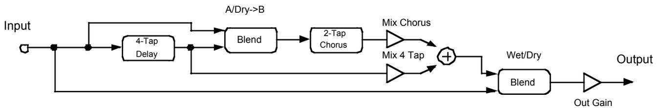
Figure 10-23 An example of routing using Chorus+4Tap
