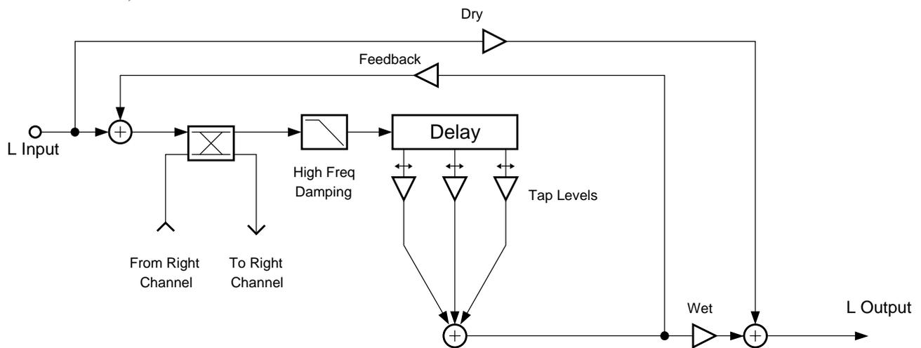
Figure 10-11 Block diagram of left channel of Chorus 2
