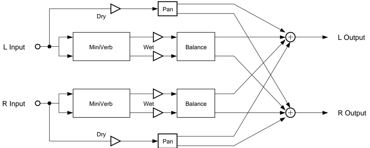
**Figure 10-2 Simplified Block Diagram of Dual MiniVerb**
