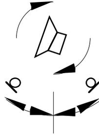
**Figure 10-41 Rotating speaker with virtual microphones**
