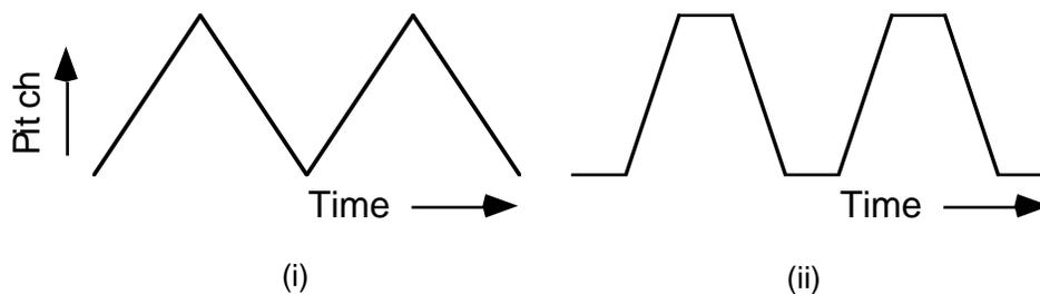
**Figure 10-16 Pitch Envelopes (i) Triangle and (ii) Trapzoid**
