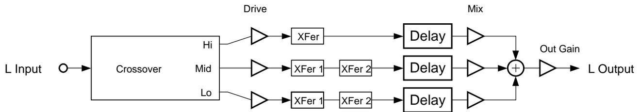
Figure 10-88 One channel of 3 Band Enhancer
