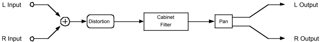
Figure 10-37 Block diagram of MonoDistort + Cab
