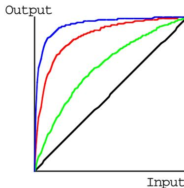
Figure 10-38 Input/Output Transfer Characteristic of Soft Clipping at Various Drive Settings
