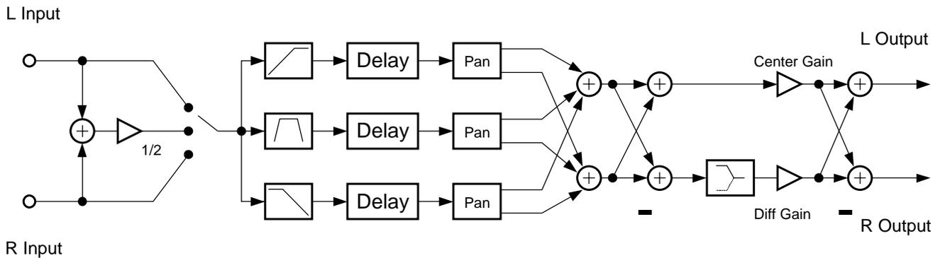
**Figure 10-95** Block diagram of Mono -> Stereo effect.
