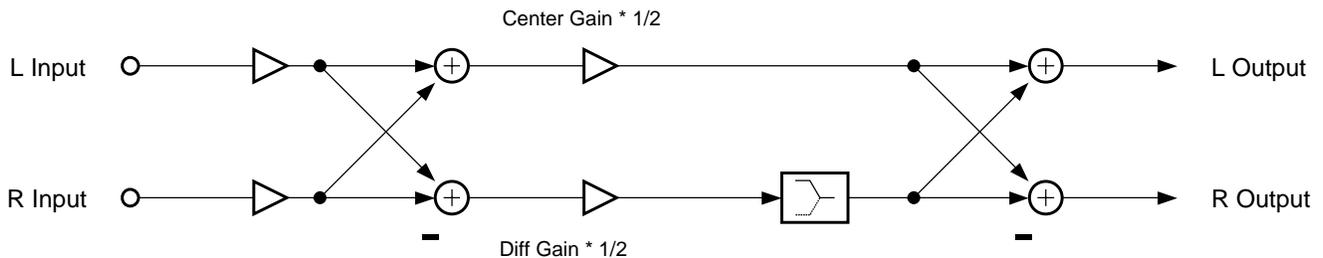
**Figure 10-94** Block diagram of Stereo Image algorithm
