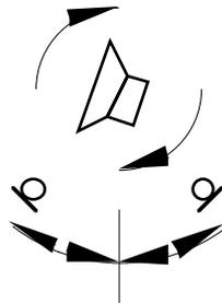
**Figure 10-44** Rotating speaker with virtual microphones
