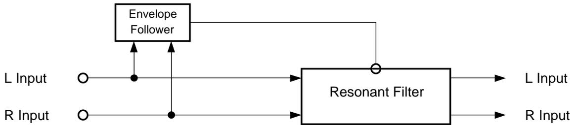
**Figure 10-50** Block diagram of envelope following filter
