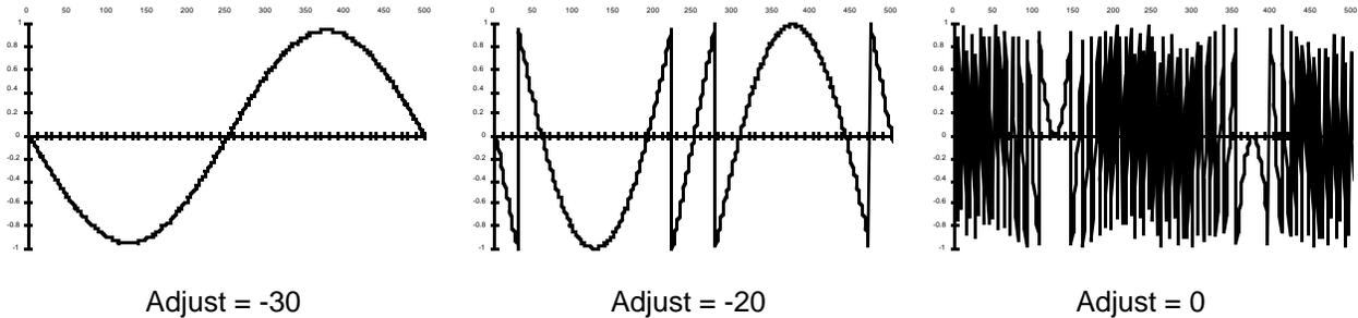
The following three graphs show the effect of WRAP on a sawtooth wave at the same frequency.
