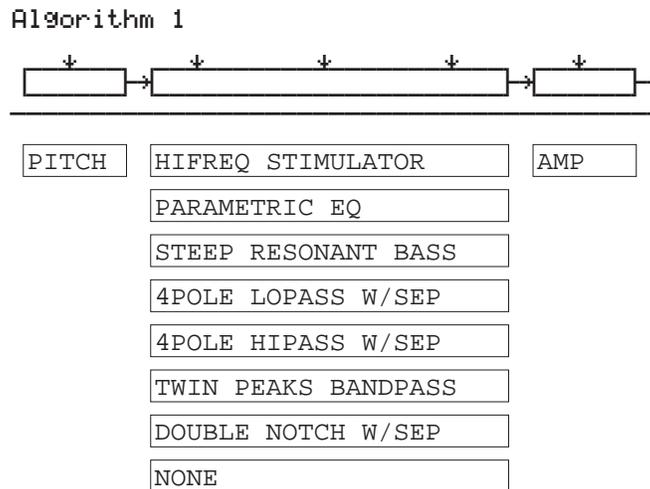
Notice that PITCH is the only value available for the first block, and AMP is the only value available for the last block. The center, three-stage block, however, allows you to choose from seven DSP functions. An eighth value, NONE, deactivates the block.
