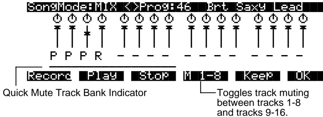
Use the M 1-8 / M 9-16 soft button to toggle between banks of eight tracks, either 1 through 8 or 9 through 16. When you press this soft button, the horizontal bar will reposition itself below the affected tracks. The table below shows the K2vx's mode buttons, and which tracks they will mute when you are playing a song:
