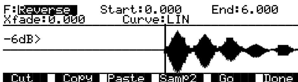
With this function you can reverse the order of the individual samples between the start and end positions you set. The Xfade parameter lets you apply a crossfade to the start and end of the reversed segment. The Curve parameter lets you select a crossfade curve. The available
