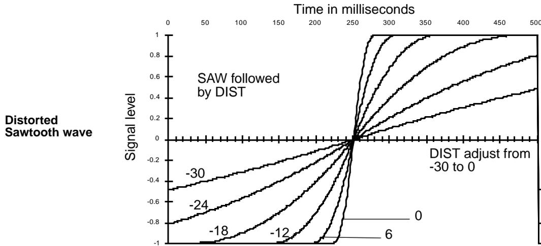
Using this function is much like overdriving an ordinary keyboard or guitar amplifier. The input signal is multiplied by the gain control (the combined values of the parameters on its control input page labeled DRV, for Drive), then passes into a distortion mapper. Large Adjust values will cause serious amounts of distortion.
