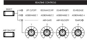
Use the [SELECT] key to select realtime controller mode A/B/C, and use knobs [1]–[4] to control the tone, effects, MIDI control changes, and arpeggiator etc. while you perform. (©p.24, 26)
