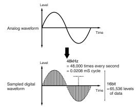
The "fixed intervals" mentioned above are generally expressed as the "sampling frequency." 48 kHz (kilohertz) means that sampling is performed 48,000 times each second, and that the interval is 1 (second)/48,000 (times) = approximately 0.00002083 (seconds) = approximately 0.02083 mS (millisecond). The higher the sampling frequency is, the closer to the original analog signal the waveform in memory will be.
