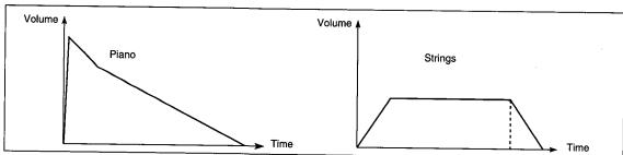
The volume changes shown in the above illustrations are called envelopes. In an N264/N364 Program, an Envelope Generator (EG) is used to create these volume-over-time changes. The VDA (Variable Digital Amplifier) uses the EG parameters to control its volume.
