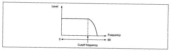
With the cutoff frequency set to 99, no high-frequency components are filtered. The filter allows you to create sounds far removed from the original Multisound.
