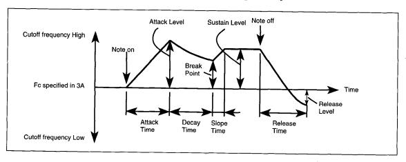
Just like a real musical instrument, the tonal quality of a Multisound changes over time. The VDF EG allows you to shape a Multisound even more, making the VDF EG an important sound building block. Unlike the VDA EG, the VDF EG has a Release Level and Time parameters, and all level parameters can be set to negative values.
