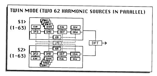
As you can see, the Twin mode provides two parallel and identical chains of sound-shaping components. These chains are called Sound Source 1 and 2 (S1 and S2) respectively. Each Sound Source consists of the following:
