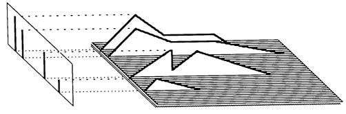
MAX: (Maximum Segment) This allows you to select one segment of each envelope as the highest point (maximum value) in that envelope. It is then set to a fixed value of 31. The Maximum Segment in each Envelope is indicated by an \* in the Level column of the appropriate segment. So you know that \* always equals 31.
