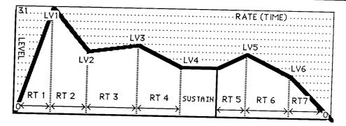
The other difference between this and the other Envelope Generators is the RTMOD (Rate Modulation) column, which can be set to ON or OFF for each segment. When ON is selected for any segment(s), the specified RATE for that segment can be increased or decreased by any of the controllers (AT VEL, RL VEL, KS) you selected on the DDA Page (4.9 above). Thus, you can vary the Attack, Decay, Sustain or Release times of your sound based on how you play the keyboard.
