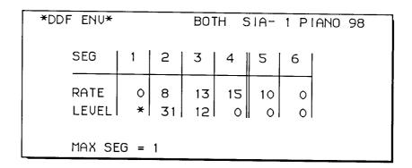
To access the DDF ENV page (DDF Envelope), press the ENV button (7) while in edit mode. In layout and function, the DDF Envelope Generator is identical to the DHG ENV. In this case, however, the envelope affects filter cutoff frequency.
