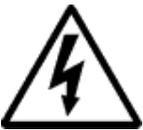
This symbol, wherever it appears, alerts you to the presence of uninsulated dangerous voltage inside the enclosure – voltage that may be sufficient to constitute a risk of shock.
