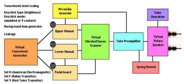
There is a "virtual tonewheel generator" which constantly plays 91 waveforms. When you depress a key, a connection matrix decides which "tonewheels" have to
