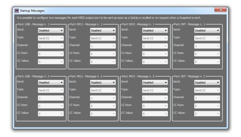
For each of the four available MIDI Output Ports it is possible to pre-configure two different messages that can be sent under a specific circumstance. The start-up messages can either be disabled or can be sent in one of the following occasions:
