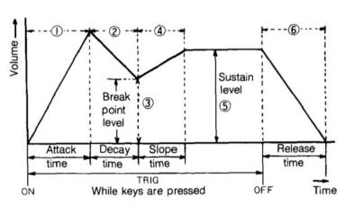
ADBSSR envelope – the diagram right is ripped from the original *Poly-800* Owner's Manual.
