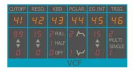
The VCF has its own DEG and offers positive or negative envelope modulation. Triggering modes of
