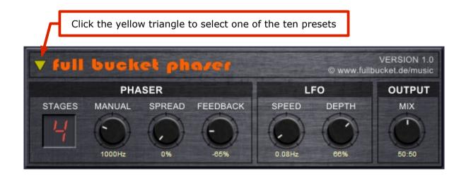
The "LFO" section controls the speed (up to 25Hz) and the depth of the low frequency oscillator modulating the Phaser frequency. The mix between original and effect is set in the "OUTPUT" section.
