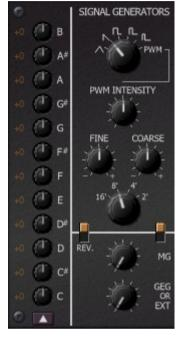
An interesting feature is the *micro-tuning* option. Each of the 12 keys can be tuned individually, allowing for other (not necessarily well-tempered) tunings like *Pythagorean* or *Wendy Carlos' Super Just* tuning etc. The small button at the bottom of the tuning knobs opens a menu with 14 predefined micro-tuning templates. Here it is also possible to load and/or save the tuning settings from/to a Scala (\*.scl) file.
