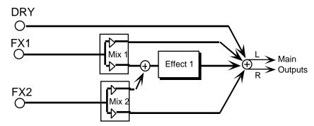
The above illustration shows the effects busses and the output mixing. Every voice is assigned to one of the three stereo busses, which go around or through the effects processing. In all of the effect routing diagrams, the heavy lines are stereo paths.
