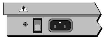
Insert the line cord into the line receptacle on the rear panel of E-Prime, next to the power switch. Plug the other end of the cable into a grounded AC outlet (the proper voltage for your E-Prime is listed on the Serial Number label on the rear panel). Turn E-Prime's power on and make sure the display lights up. If not, check your connections and power source.
