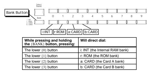
The lower {0} to {3} buttons are used to choose between i:INT, r:ROM, a:CARD and b:CARD sounds. Note that if there is no card installed, or there is no sound data on the card, the a:CARD and b:CARD banks will not be recognized.
