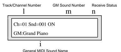
E-Prime behaves as though an enlarged 16-track sequence has been selected, and as though the current MIDI Mode=MULTI. Incoming MIDI will be received on all 16 MIDI channels, to 16 discrete inbound Track/Channels. The default effect algorithm (EQ-CHORUS + REVERB) will be installed, and all Track/Channels will be routed through the effect.
