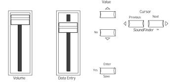
The method used to modify or edit sounds, presets, and system parameters is called Parametric Programming. This may sound complicated, but don't worry. Once you've grasped a few basic concepts, you'll find that operating E-Prime is quite simple, given its many capabilities.
