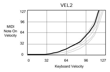
• PIANO/SYNTH VEL2 — Dark line (thicker) is VEL2. Slightly harder key strikes are required for average playing, but this still allows a softer touch to reach maximum velocity levels.
