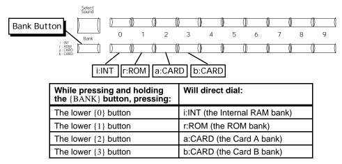
When pressed in Select Sound and Replace Track Sound modes, the {BANK} button transmits MIDI Bank Select messages corresponding to the Sound bank you selected.
