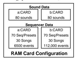
Both sounds and sequencer data stored to a RAM card can be played directly from the card (when it's properly inserted into the card slot on E-Prime). Each Preset/Seq/Song bank is a world unto itself: for example, songs can only be constructed of sequences from the same bank. The Preset/Seq/Song banks are sized as follows:
