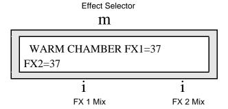
Changing this parameter causes a new algorithm to be selected, which in turn changes the types of parameters that will be available on the rest of the sub-pages. Selecting a new effect algorithm will automatically set all the effect parameters to their default values for the new effect. The available effects are:
