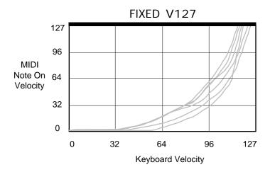
• FIXED V127 — This setting is also a fixed velocity curve, with full volume. This is good for playing drum/percussion parts when you want a part without dynamic changes.
