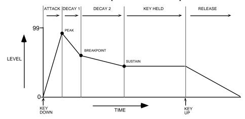
Although the envelope shape in the above illustration is the most commonly used (a rise followed by decays), other shapes are possible. For more information on the specific envelope parameters, see  $Section\ 6$  —  $Standard\ Sound\ Parameters$ .
