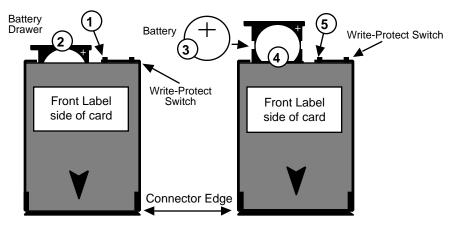
**Tip:** If you replace the battery while the card is plugged into E-Prime, with E-Prime's power on, you will not lose the data on the card. Do not turn off E-Prime's power while the card is installed with the battery removed, or card data will be lost.
