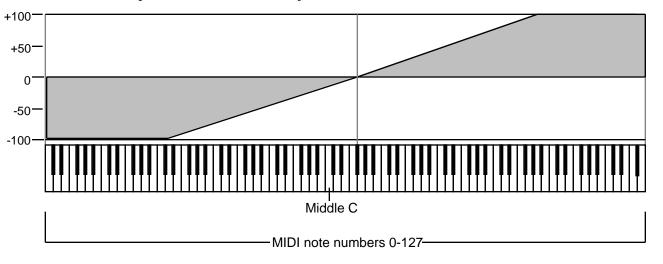
As the above illustration shows, the effect of KEYBD as a modulator goes negative as well as positive. The effect of KEYBD is to reduce the manual level on notes below the break point (F# above Middle C, F4+, MIDI Note #66), and increase the manual level on notes above the break point. Negative modulation amounts will do the opposite.
