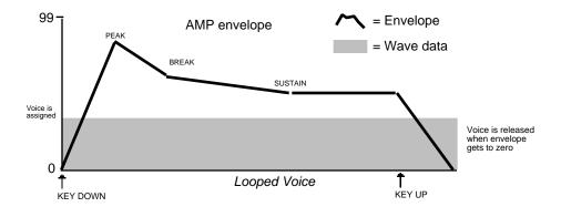
For a sustaining wave, when the envelope mode = FINISH:
