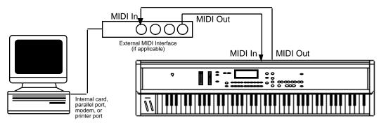
Computer (with MIDI Interface) connected to E-Prime's Keyboard
