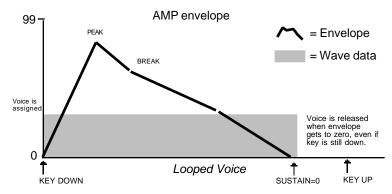
For unlooped, non-sustaining, waves (specifically those in the Percussion and Drum categories) the voice becomes free as soon as the sample has played through to the end, no matter where the envelope level is. The voice is released and is available for use by other sounds:
