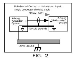
Fig. 1 depicts a system interconnection where a ground loop can exist. Fig. 2 depicts a system interconnection where a ground loop does NOT exist. When interconnecting 3-prong grounded systems, you can use signal isolation transformers to prevent ground loops. This coupling transformer effectively isolates two interconnected system signal grounds, while still allowing the signal to pass through.
