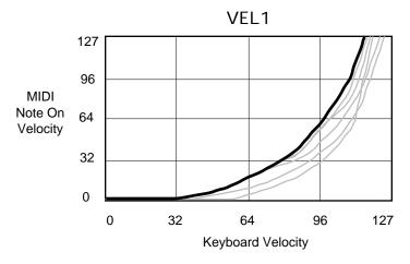
• PIANO/SYNTH VEL1 — Dark line is (thicker) VEL1. This is for someone with a light touch. On this setting, it is easier to reach the maximum level of any velocity controlled parameter.
