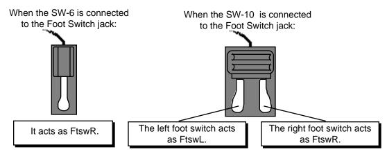
The FtswL and FtswR parameters on System • MIDI page 2 allow you to reassign the foot switches to a variety of functions, including sostenuto and stopping/continuing the sequencer. See Section 2 — System • MIDI Parameters for more information.
