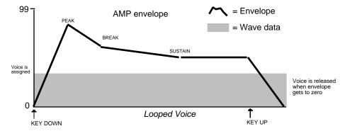
For a sustaining wave, when the envelope mode = FINISH:
