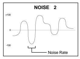
The Noise Rate defines how frequently the levels will change. Low values will cause levels to change very slowly; with high values the levels will change quickly. A rate value of zero will select a different random level with each key down, but the level will not change for as long as the key is held.
