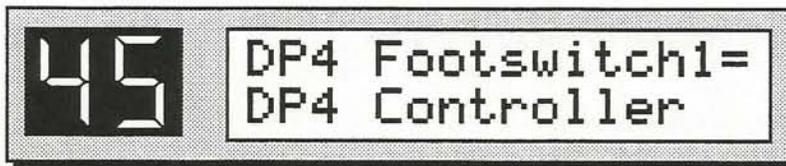
2. Using the **Data Entry Knob**, set the DP/4 Footswitch 1 to "DP4 Controller." This allows the foot switch to be used as the modulation source.
