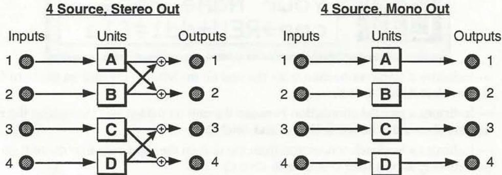
Input 1 is a mono input to Unit A; Input 2 is a mono input to Unit B; Input 3 is a mono input to Unit C; and Input 4 is a mono input to Unit D.
