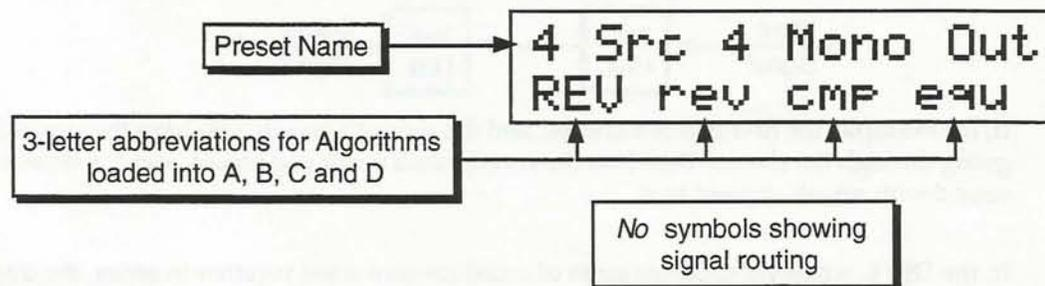
Note that there are no signal routing symbol between A, B, C, or D. This shows that all four units are functioning independently, not connected in any way.
