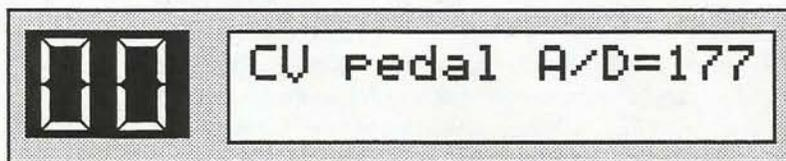
This read-only parameter displays the current control voltage reading of the CV Pedal input's 8 bit analog-to-digital converter. With a CVP-1 pedal connected, the typical range is 000 to 177, with the fully up position showing 000 and fully down showing approximately 177.
