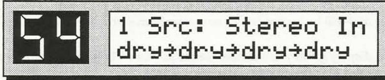
3. Press **Select** again. This loads the Config Preset, changing the current Config type to 1 Source, and loading all 4 Units with the Dry (No Effect) algorithm. The DP/4 automatically sends you to Unit A.
