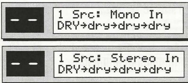
The LED Display will "turn off" the preset number when it is invalid. This will happen whenever you change settings or parameter values. For a more in-depth discussion on Config Presets, and a thorough explanation of all of the parameters associated with Config Presets, see *Section 3 — Config Parameters*.
