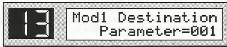
7. Here you select which parameter in the algorithm will be modulated by the selected controller. Since Wet/Dry Mix is parameter 01 in *every* algorithm, set it to "Mod1 Destination Parameter=001."
