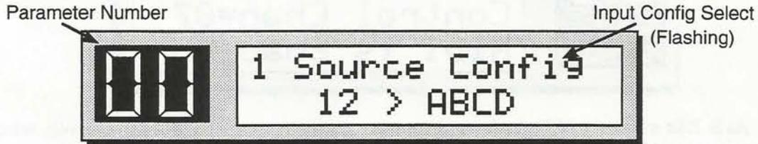
The LED display should indicate parameter 00, which is the *Input Config Select* parameter, and the current config type should be flashing in the upper line of the LCD display. (If not, press the **Left Arrow** button until this is the case.)
