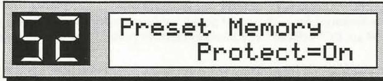
3. If the word "On" is flashing, move the **Data Entry Knob** counterclockwise to the "Off" position. If the word "Off" is flashing, RAM preset data can be changed.
