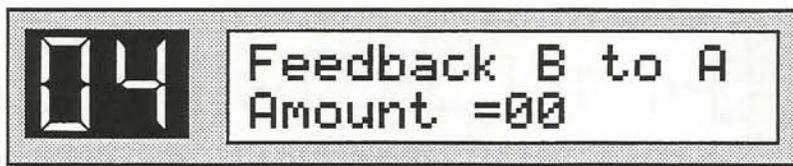
This screen allows you to control a feedback signal from Units B to the front of Unit A. A setting of 00 would not allow the feedback signal back into the units, whereas a setting of 99 would permit a full feedback signal.
