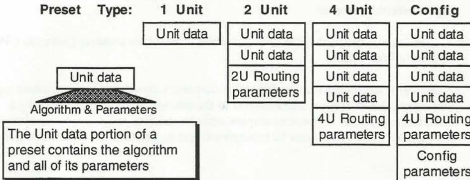
There are 400 presets in the DP/4; 100 presets (storage locations) for each type of preset. The first 50 presets (00 to 49) are user programmable (battery backed up RAM). Presets 50 to 99 are ROM factory presets. These groups of 50 presets are referred to as *Preset Banks*.
