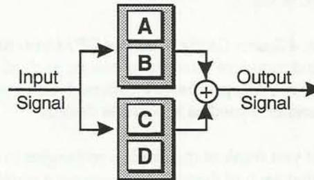
Any combination of serial and parallel routing can be chosen, both *within* the pairs and *between* the pairs of units. This allows a huge variety of different configurations, each of which will sound distinctly different.
