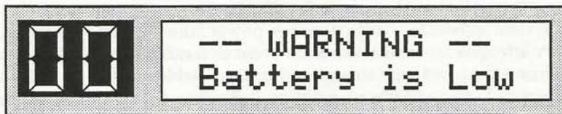
This will only appear for a fixed period of time, and then you can commence with normal operation. Make sure that all RAM configs, presets and system parameters are saved, and take the DP/4 to an Authorized ENSONIQ Repair Station as soon as possible to have the battery replaced.
