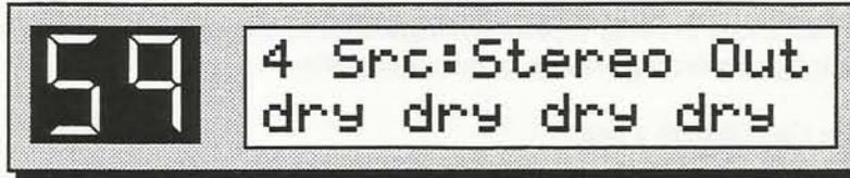
3. Press **Select** again. This loads the Config Preset, changing the current Config type to 4 Source, and loading all 4 Units with the Dry (No Effect) algorithm. The DP/4 automatically takes you to Unit A.
