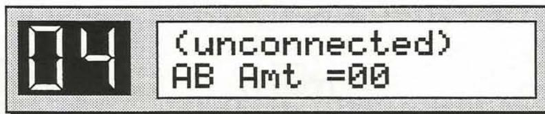
This parameter does nothing because of the nature of a parallel connection, there is no dry path (or feedback) around the units.
