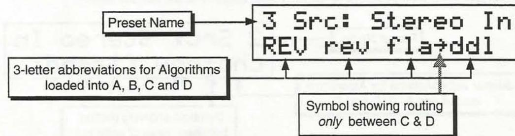
Note that there is no signal routing symbol between A and B or between B and C. This shows that there is no connection between the A, B, and CD Units.
