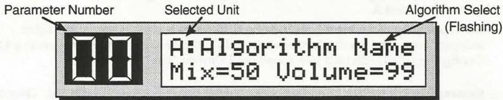
The LED display should indicate parameter 00, which is the *Algorithm Select* parameter, and the algorithm name should be flashing in the upper line of the LCD display. (If not, press the **Left Arrow** button until this is the case.)
