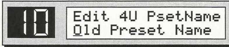
At this point you can name your "ultimate preset." The **Left** and **Right Arrow** buttons will move the cursor left and right, and the **Data Entry Knob** will change the alphanumeric characters. For more about this, refer to *Section 7 — Storage*.
