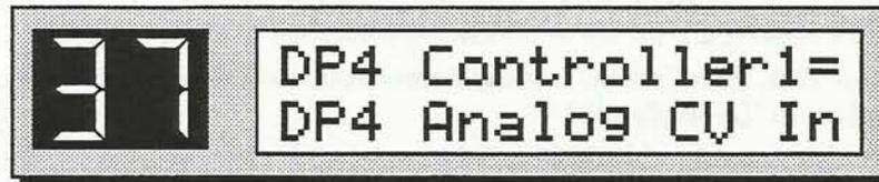
2. Set the "DP4 Controller1" parameter to "DP4 Analog CV In" as shown above (you will use this and the next seven parameters to define the eight controllers the DP/4 will recognize as modulators).
