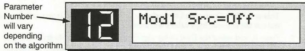
5. Set the parameter to "Mod 1 Src=Cntrl 1." The lower line of the display shows the name of the controller that has been selected as "Cntrl 1" in System•MIDI mode. It should read "DP4 Analog CV In."
