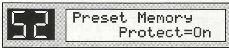
3. If the word "On" is flashing, move the **Data Entry Knob** counterclockwise to the "Off" position. If the word "Off" is flashing, you can save your new preset.
