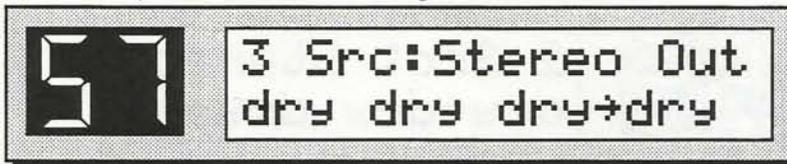
3. Press **Select** again. This loads the Config Preset, changing the current Config type to 3 Source, and loading all 4 Units with the Dry (No Effect) algorithm. The DP/4 automatically takes you to Unit A.
