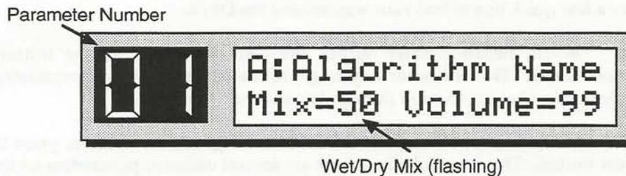
The LED display should indicate parameter 01, which is the Wet/Dry Mix, and the mix value should be flashing (if not, press the **Left** or **Right Arrow** button until this is the case).
