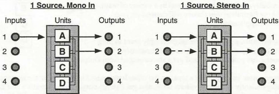
In the first example, the signal present at Input 1 will be fed as a mono signal to all four units. In the second, the signals present at Inputs 1 and 2 will be fed to all four units as a stereo signal. (Remember, a single *source* can be mono or stereo.)
