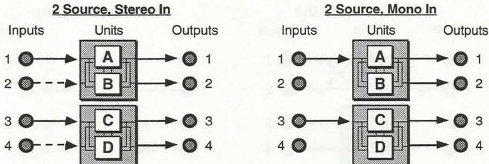
In the first example, the signal present at Inputs 1 and 2 will be fed as a stereo signal to Units A and B. The signal present at Inputs 3 and 4 will be fed as a stereo signal to Units C and D. In the second example, the signal present at Input 1 will be fed as a mono signal to Units A and B. The signal present at Input 3 will be fed as a mono signal to Units C and D.
