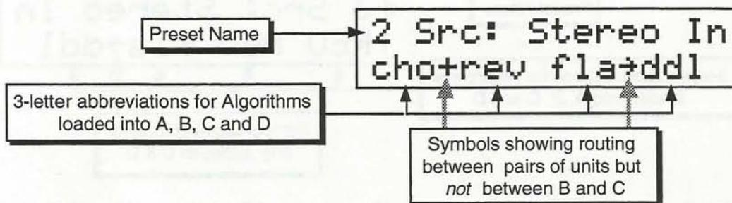
Note that there is no signal routing symbol between B and C on the lower line of the display. This shows that there is no connection between Units A & B and Units C & D.
