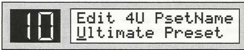
The **Left** and **Right Arrow** buttons will move the cursor left and right, and the **Data Entry Knob** will change the alpha-numeric characters at the current cursor position.
