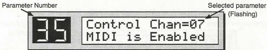
As in Edit mode, the LED display indicates the parameter number, and the currently selected parameter is flashing in the LCD display.
