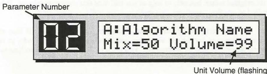
6. Move the **Data Entry Knob** to adjust the output volume of the Unit. This parameter is used to control the levels of the various units relative to each other in a preset.
