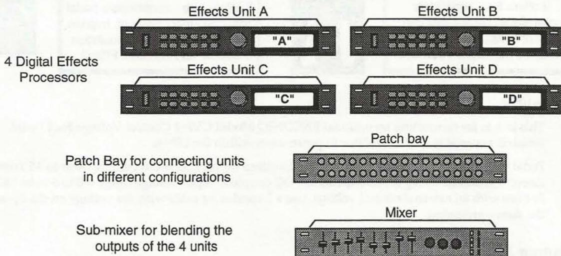
Now suppose you could change the effect in all four units, repatch the patch bay into a whole new setup, and adjust the levels on your sub-mixer, all with the press of a button (or with a MIDI program change, or a press of the foot switch). That's the DP/4.
