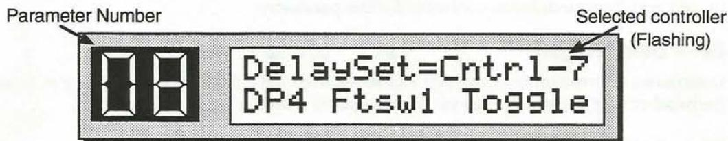
This allows you to toggle between a *recording* state and a *playback* state. In playback, it will loop on the audio which was input during the recording state (of up to 3.6 seconds).
