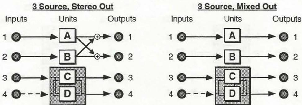
In both examples, the signal at Input 1 goes to Unit A; the signal at Input 2 goes to Unit B. The signal at Inputs 3 and 4 is fed as a stereo signal to Units C & D. In the first example, the stereo outputs of units A and B are digitally mixed together and sent to Outputs 1 and 2. The stereo output of the CD pair goes to Outputs 3 and 4.
