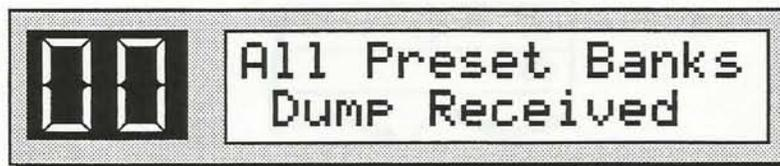
The top line of this message will describe the type of dump received. The preset type and number are shown for single preset dumps. Only the type is shown for preset bank dumps. Dumps containing system parameters will have an additional message which follows the confirmation message to indicate that the previous settings of the system parameters have been replaced by new data.
