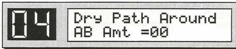
This screen allows you to control an external dry signal around Units A and B. A setting of 00 would not allow a dry signal around the units, whereas a setting of 99 would permit a full signal around the units.
