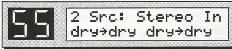
3. Press **Select** again. This loads the Config Preset, changing the current Config type to 2 Source, and loading all 4 Units with the Dry (No Effect) algorithm. The DP/4 automatically takes you to Unit A.
