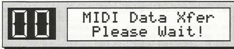
When the dump is complete, the following message will appear for a moment to indicate that the transmission occurred without errors.
