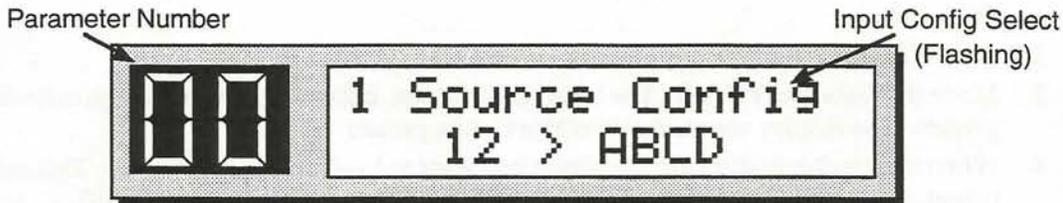
The LED Numeric Display should indicate parameter 00, which is the *Input Config Select* parameter, and the current config type should be flashing in the upper line of the LCD display (if not, press the **Left Arrow** button until this is the case).
