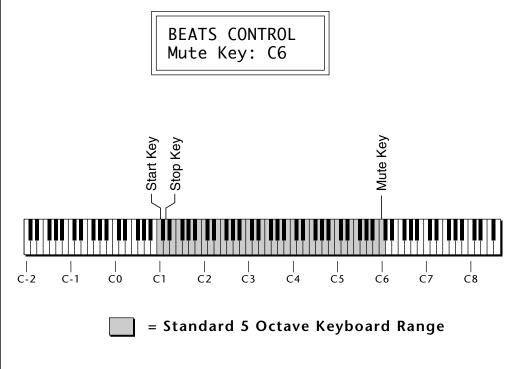
Control keys can be placed out of the way at the ends of the keyboard or anywhere you prefer.
