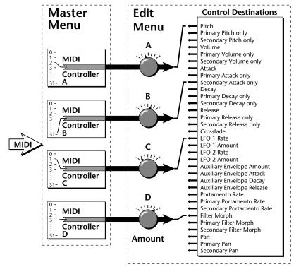
The MIDI controllers A-B-C-D must have both a source (0-31), and a destination assigned.
