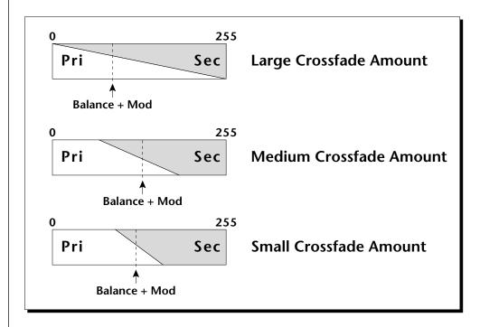
Modulation and Crossfade Balance are **added** together to determine the mixture of primary and secondary instruments. Higher values increase the secondary volume.
