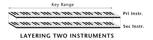
This diagram shows how instruments can be layered or "stacked" using the primary and secondary instruments.
