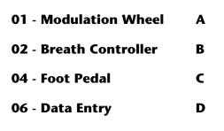
To complete the connections for a particular preset, go to the Edit menu, Realtime Control, and route the MIDI A, B, C, D to the desired destinations. These could be patched to any 4 destinations or even to the same destination. The MIDI Controller Amount menu, (in the Edit menu) allows you to scale the amounts of each of the controllers by a positive or negative value. The signal flow is shown in the diagram below.
