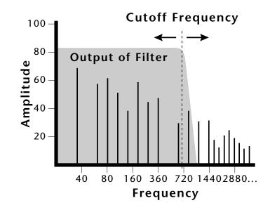
The point at which the frequencies begin to be cut is called the **Cutoff Frequency** (or Fc for short). A filter that let only the high frequencies pass would be called a High Pass filter. Using a filter, we now have a way to control the harmonic content of a sampled sound. As it turns out, a low pass filter can simulate the response of many natural sounds.
