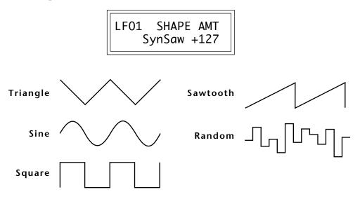
The Triangle, Sine, Sawtooth and Square LFO shapes can also be **Synced**to the Beats tempo or to external MIDI clock. The LFO waveforms preceded by "Syn" are synced LFO's. With the LFO synced to the beats tempo, the LFO rate will follow any changes in the beats tempo.
