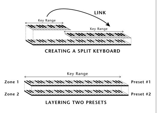
These diagrams show how keyboard splits and layers can be created by linking presets. Remember that each preset can consist of both a primary and secondary instrument. Orbit has an extensive modulation implementation using two multiwave LFO's (Low Frequency Oscillators), two envelope generators and the ability to respond to multiple MIDI controllers. You can simultaneously route any combination of these control sources to multiple destinations.
