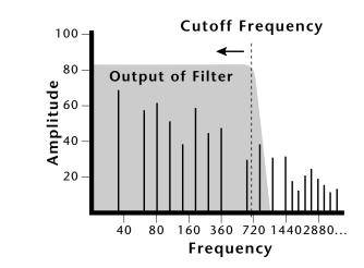
Open the filter back up to 255, then move the cursor underneath the Q. Set the Q to 10, then move the cursor back under the Fc. As you change the Fc, notice that the sound now has a sharp, nasal quality. With a high Q, frequencies at the cutoff frequency (Fc) are being boosted or amplified.
