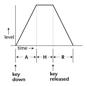
If the key is released during the Hold (H) phase, the Release phase begins.
