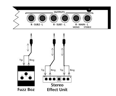
Using the programmable outputs and returns, specific presets can be routed through your favorite effects without using up precious mixer channels.
