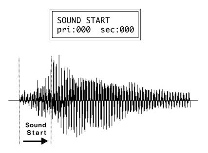
The Sound Start parameter allows you to cut off the beginning of the sound. Higher values move the start point toward the end of the sound.
