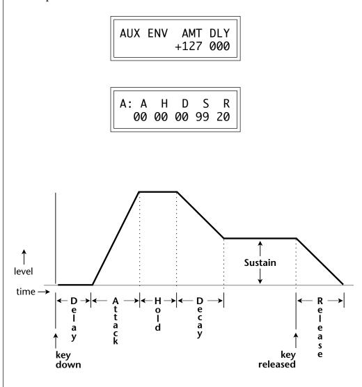
This diagram shows the six stages of the Auxiliary Envelope Generator.
