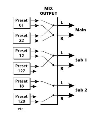
Each preset can be routed to one (and only one) set of stereo outputs.
