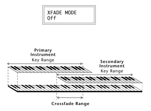
••• To use the keyboard for crossfade, set the Crossfade Balance to 64 and the Key Center to the split point.
