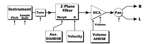
The **Tone** filter is a simple tone control and can be used to brighten or darken the tone of an instrument. Each of the 17 Z-plane filters is a powerful synthesizer filter which can dramatically alter the sound of an instrument.
