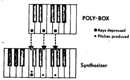
Now, if the pitch of the controlling oscillator is lowered to F below middle C  $(F_3)$ , the Poly-Box automatically transposes and produces the notes:
