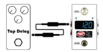
If you are sending taps to a Boss pedal, then you should configure its output to *normally-closed* using the Setup menu. If you are sending taps to the *EXP* jack of a Strymon pedal, then you will need to use a TRS cable and set its output to *Pull-up* using the DIP switches inside the SMARTClock.
