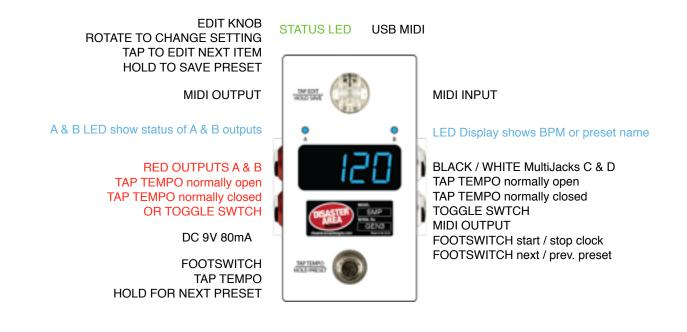
**USB MIDI:** The SMARTClock firmware allows the USB port to function as a MIDI interface for your compatible PC, Mac, or iPad (using the Apple Camera Connection Kit). The SMARTClock will receive and send MIDI messages over USB for device control.
