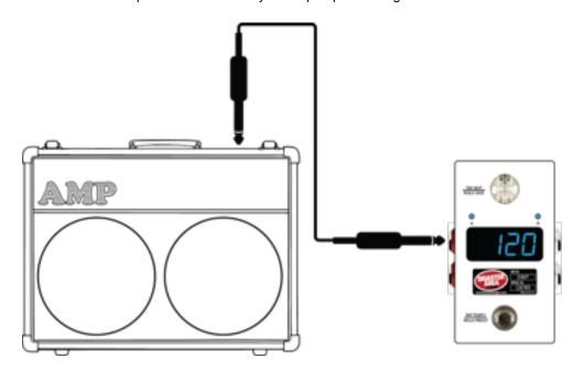
If your amplifier uses a TRS / stereo jack for function switching then you can use a stereo y-cable to connect more two SMARTClock outputs together. If you're controlling a Strymon pedal, you'll need to set your output's DIP switch to enable the *pull-*up and to connect with a TRS cable.
