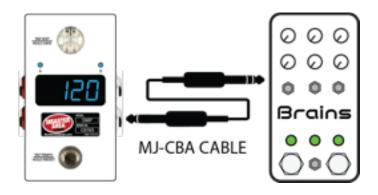
Chase Bliss Audio pedals require the use of the Disaster Area MJ-CBA cable. Empress and Meris devices can use a standard mono / TS patch cable. Please consult the manual for your pedal for information on how to configure it to use MIDI.
