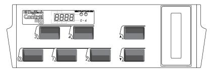
The Program Number/Continuous Controller/MIDI Channel display is a 4-digit LED display. The pedals perform the program change and bank up/down functions and can be used as continuous controllers. The back of the unit has a standard 5-pin DIN MIDI jack and a 3.5mm Power In jack.
