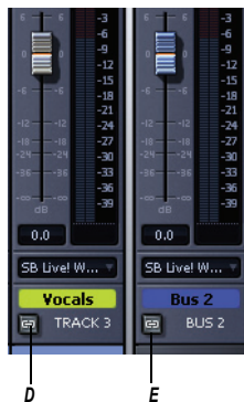
A. A track strip selector in the Track view B. A track selector in the Track view C. A bus strip selector in the Track view D. A track strip selector in the Console view E. A bus strip selector in the Console view
