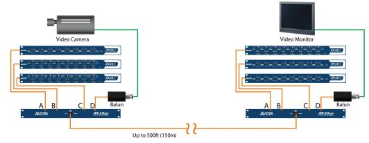
Figure 3. Video can be transmitted over Cat-5e with the use of Aviom's AN-16SBR System Bridges, which are used in pairs to combine multiple Pro16 data streams, as well as video, over a single cable.
