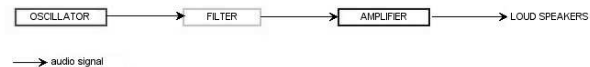
Basic audio path in analog synthesis
