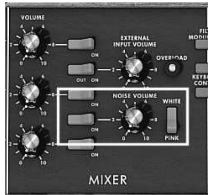
The noise generator set on the mixer
