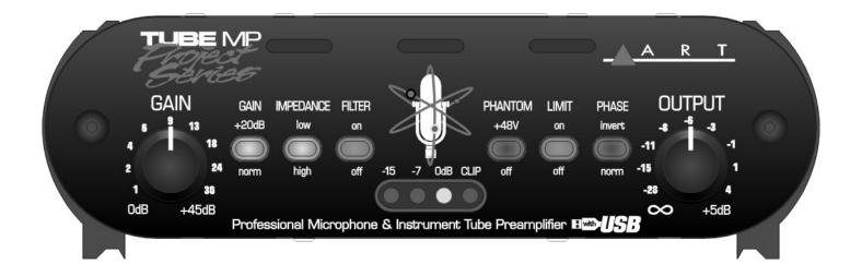
The **Gain** Control directly adjusts the input amplifiers giving you control over the dynamic range of your source. You get a 45dB gain range when using the XLR input and a 25dB gain range when using the ½" input. Set the control counterclockwise to minimum gain when connecting the inputs.
